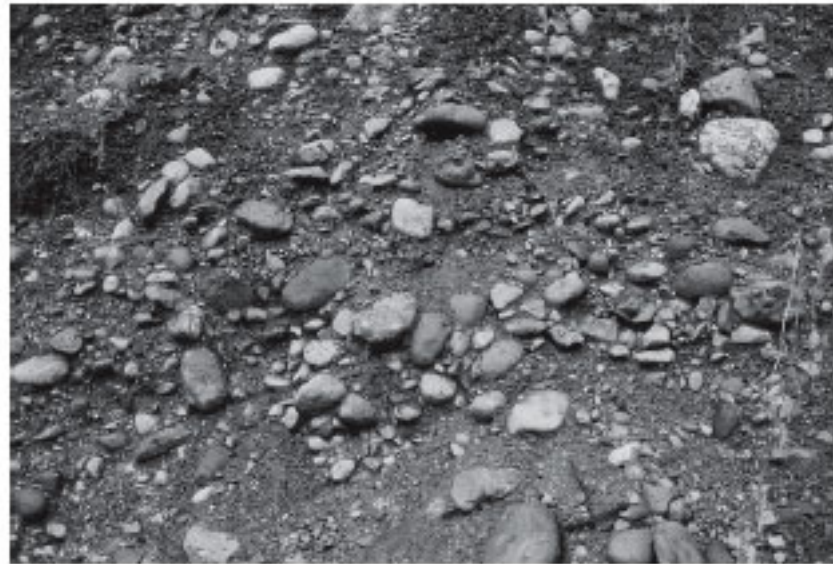
FIG. 16. Poorly-sorted matrix supported gravels of Facies 1.
